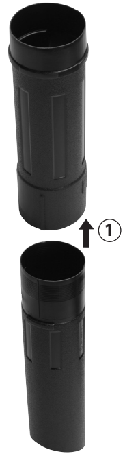
Figure 3-8: Connecting lower and upper vacuum tube together
